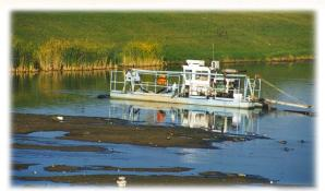
**P** arker Ag Services dredges sediment from biosolids lagoons, silt retention ponds, manure ponds, drinking water sludge settlement ponds, and aerated lagoons. This neat and clean dredge operation minimizes odor, since the solids are not exposed to the air.
